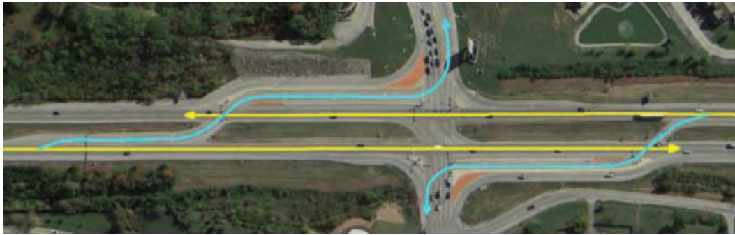
Continuous Flow Intersection (aka DLT)
